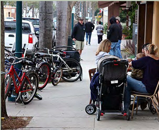
Sidewalks have three parts: the shy zone, the furniture zone and the walk-and-talk zone.
