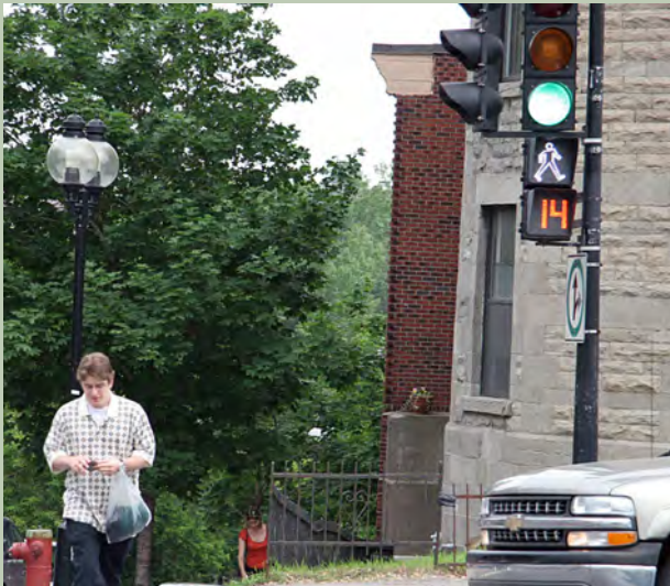
Signals should recall to WALK during the cycle and instruct pedestrians on crossing times.
