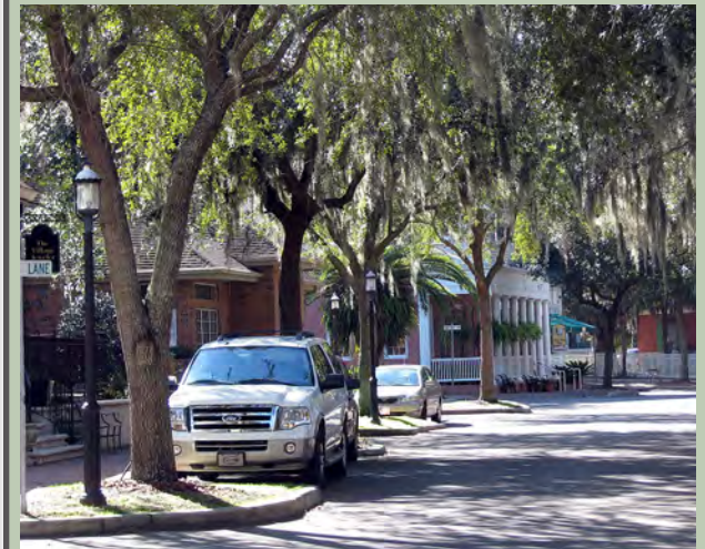
Tree wells in the Town of Tioga, FL, provide shade and inset parking.
